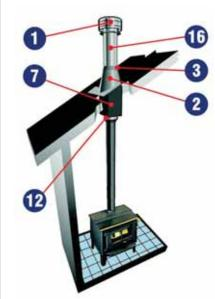
Note: If your chimney runs more than 38', you must install a Roof Support \*TLCRS.
