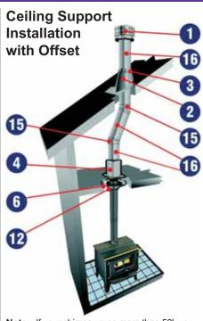
Note: If your chimney runs more than 50', you must install a Roof Support \*TLCRS.
